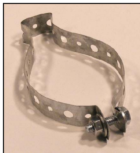
Router band clamp made of plumbing hanger tape.
